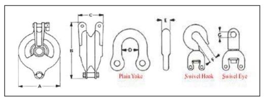
Note: The safe working load is based on a factor of safety of 4:1 of the ultimate capacity. If a higher factor is required the safe working load must be lowered accordingly. Snatch block sheaves are filtered with tapered roller bearings.
